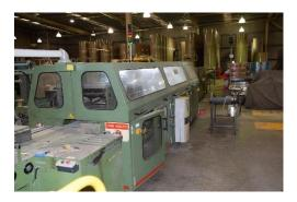
Sheeter complete with two lines for paper wrapping, labelling, ream collator, two box lines, conveyor to pallet stacker.
