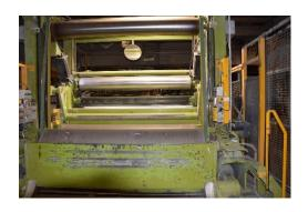
Salvage rewinder Jagenberg VariDur,width 2770mm on knife shaft, Unwind Jagenberg: inclined floor pick up, shaftless with individual disc brakes, tension control, various core chucks, 10 slitters manual setting, core feeder, shaftless rewind 1800mm diameter. Twin motor drive, reel ejector and lowering table. Year 1996, number AW236``2, TYPE 45U5 -2600.
